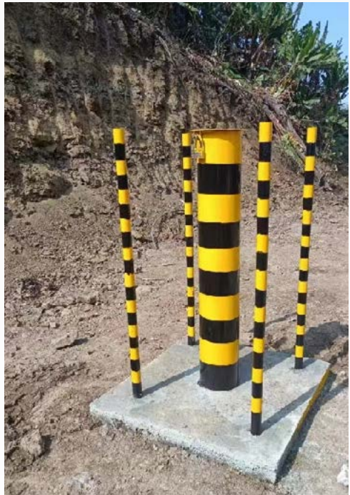
Groundwater Monitoring Well
